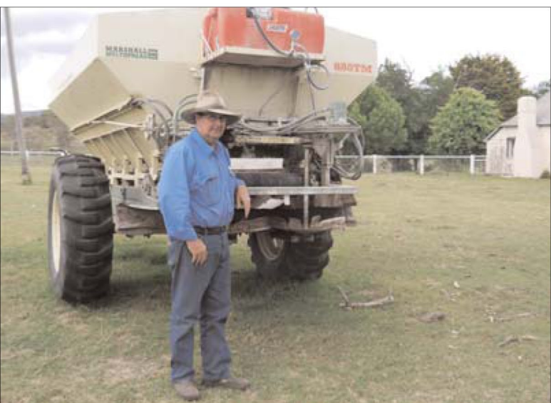
Stewart Bulmer, Bolivia Station, Tenterfield with his Marshall spreader used to apply manure treated with the Petrik biology applied through four spray nozzles.
